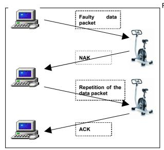
Fig 3: transmission error
